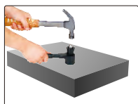
hammer impact to apply test force
